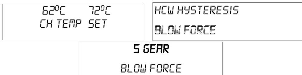
This function allows to choose the operations speed of the fan. Range of regulations is between 1 and 10 (one can assume those are the gears of the fan). The higher the gear the faster the operation of the fan, whereas gear 1 is the minimal speed and gear 10 is the maximal speed. Change of gears is being done by the means of PLUS and MINUS buttons. The fan always starts up with the maximal speed which allows it to start operation even with some amount of dust present in the engine.
