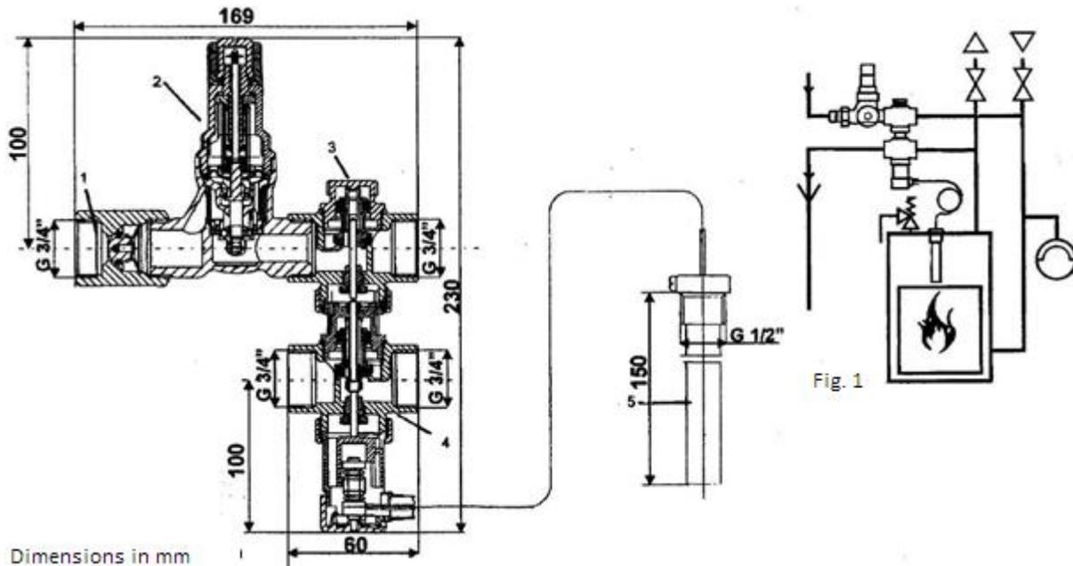
The 5067 thermal safety valve is intended for solid fuel boilers equipped with thermostatic valves in accordance to Polish Norm PN-EN303-5. It is recommended for boilers without cooling coils. Fig. 1 shows the installation method; in close proximity to the boiler it is important to lead the pipes so that there are no pressure losses.
