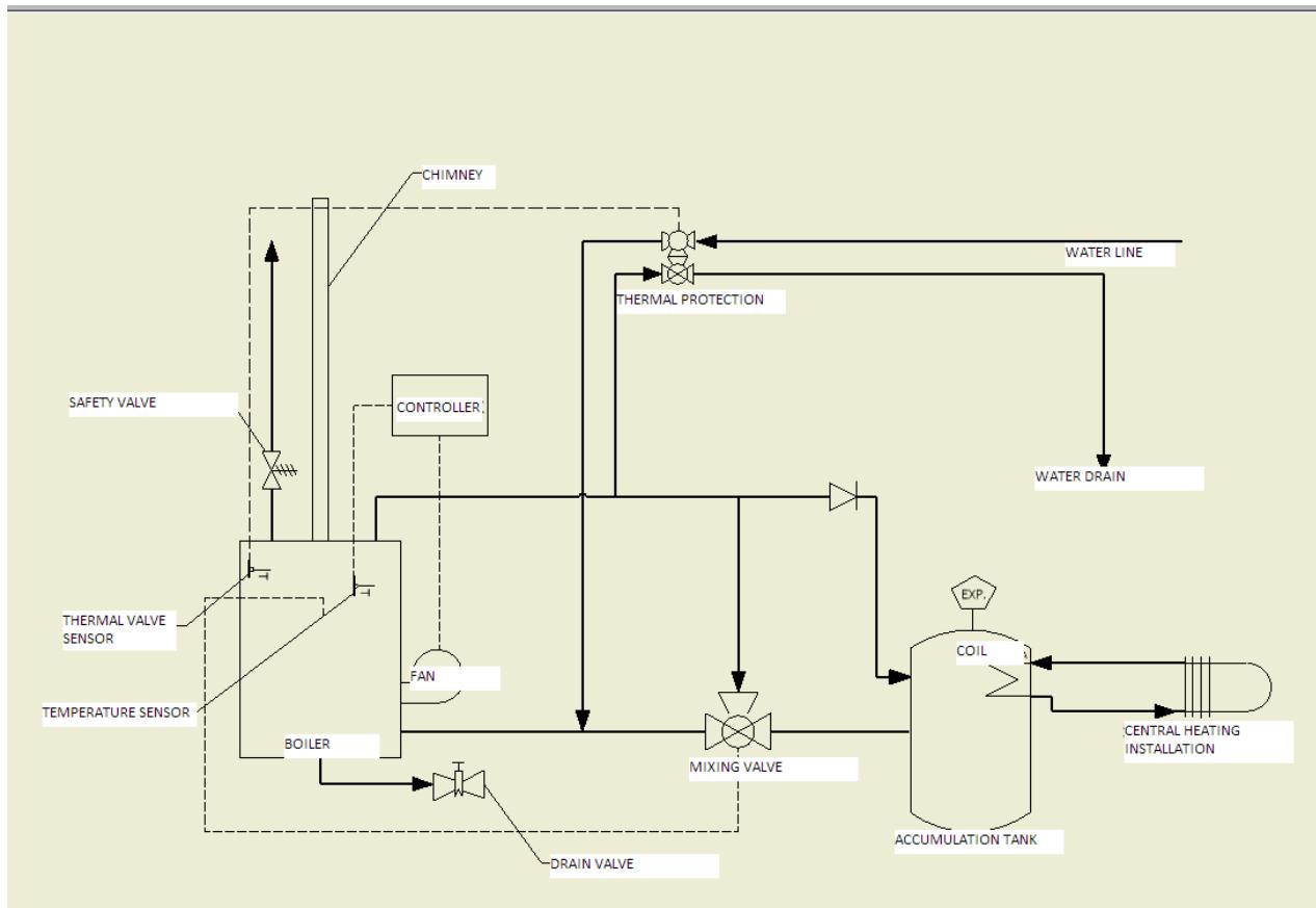
Fig. 5. Safety schematics for boilers working in sealed central heating systems.
