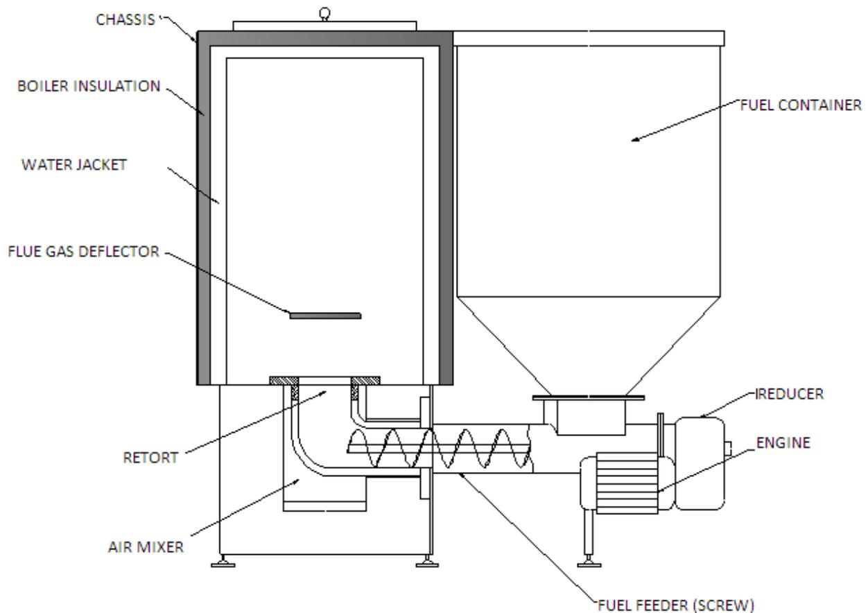
Fig. 2. Schematic diagram of the Moderator boiler.
