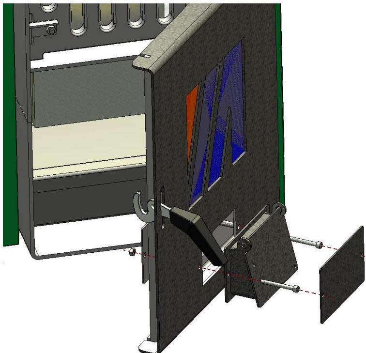
Fig. 6. - Air damper installation
