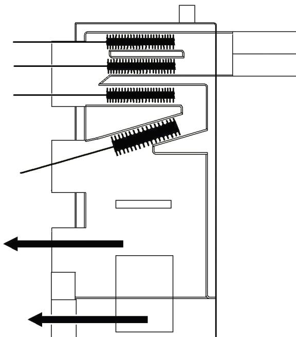
Fig. 8 Boiler (exchanger) cleaning schematics.
