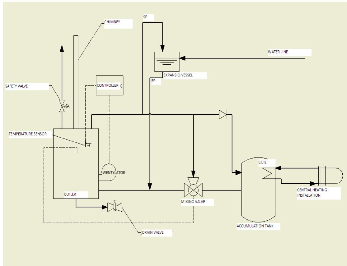
Fig. 4. Safety schematics for boilers working in open vented central heating systems.
