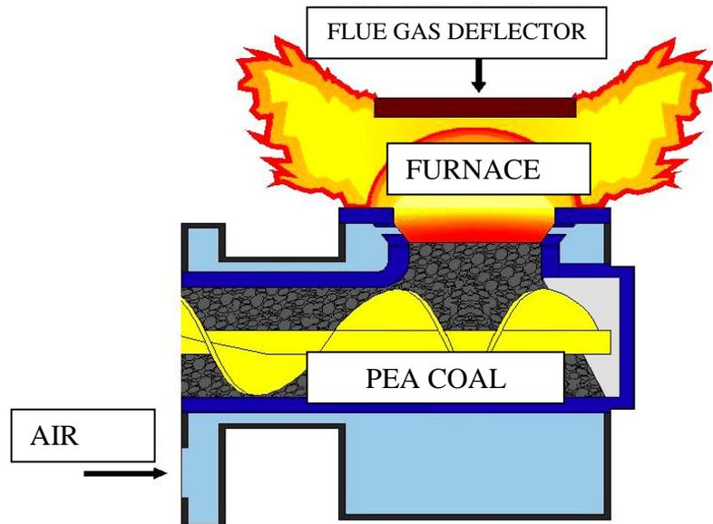
Fig. 1. Lower coal feed retort.
