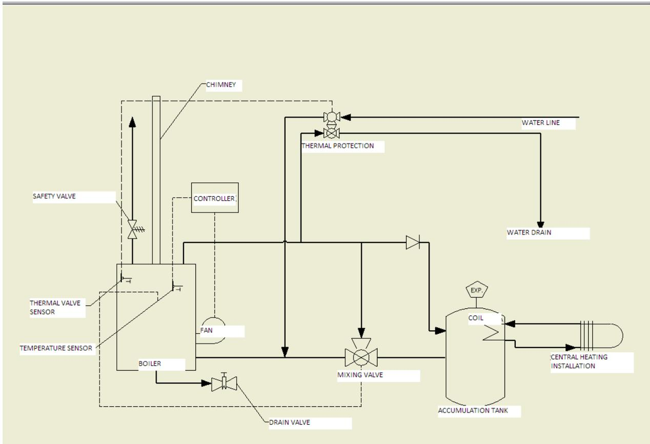
Fig. 5. Safety schematics for boilers working in sealed central heating systems.
