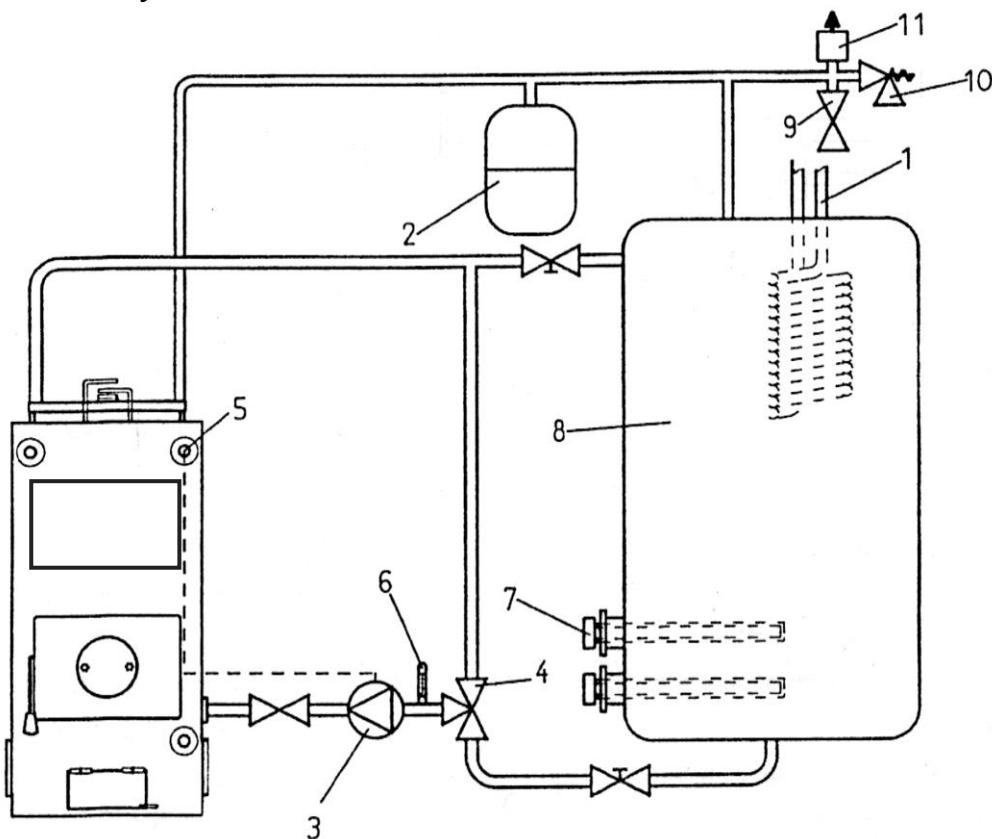
Fig. 9. **Three-way valve connection schematics**
