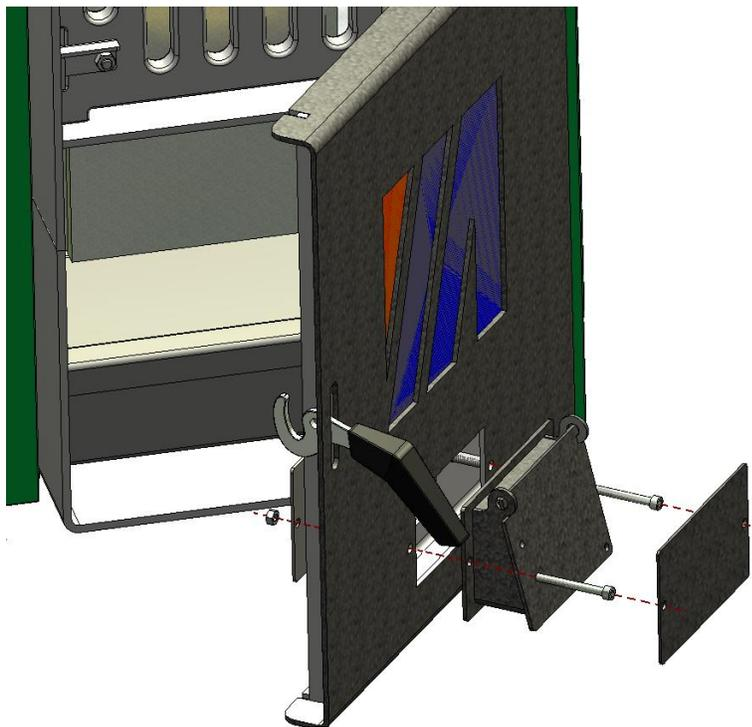
Fig. 6. - Air damper installation
