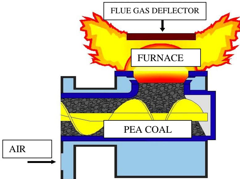
Fig. 1. Lower coal feed retort.
