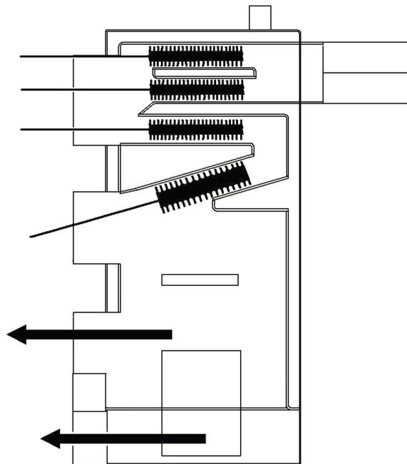
Fig. 8 Boiler (exchanger) cleaning schematics.
