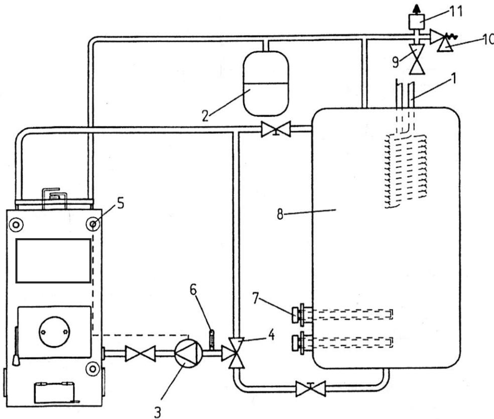
Fig. 9. **Three-way valve connection schematics**
